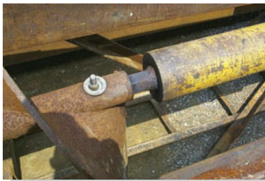
The drill shaft is connected to the soil auger using a shaft having a square cross section.
