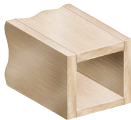
Wooden box beam
