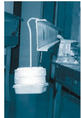
Demonstration of how a cantilever beam deflects when loaded through the centroid (above) and through the shear center (below).
