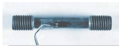
Typical steel specimen with attached strain gauge.
