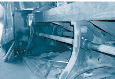
The shaft of this cutting machine is fixed at its ends and subjected to a torque at its center, allowing it to act as a torsional spring.
