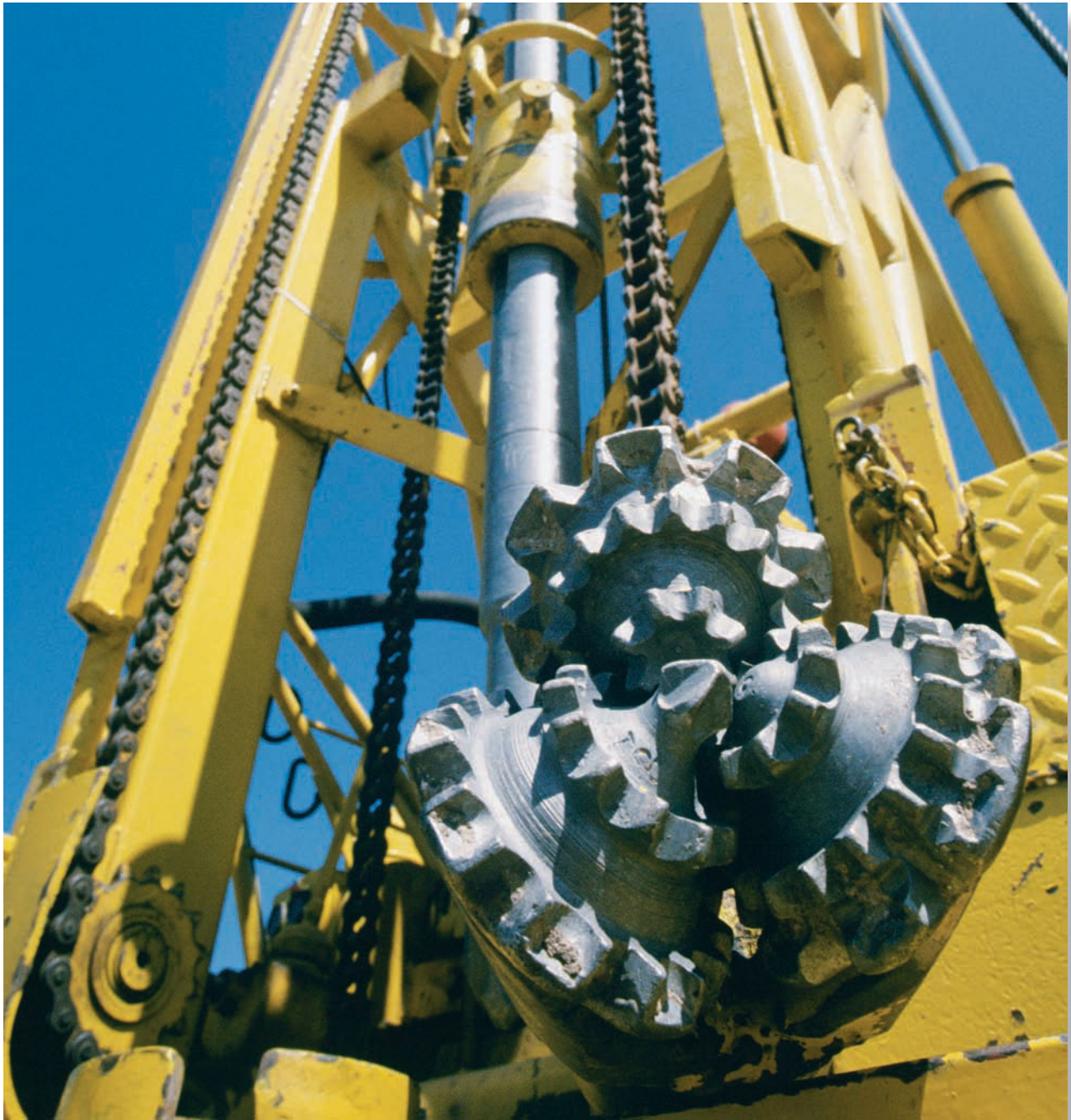
The string of drill pipe suspended from this traveling block on an oil rig is subjected to extremely large loadings and axial deformations.
