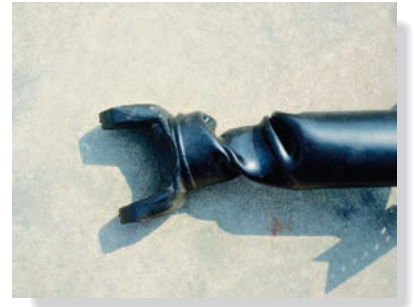
This tubular drive shaft for a truck was subjected to an excessive torque, resulting in failure caused by yielding of the material.
